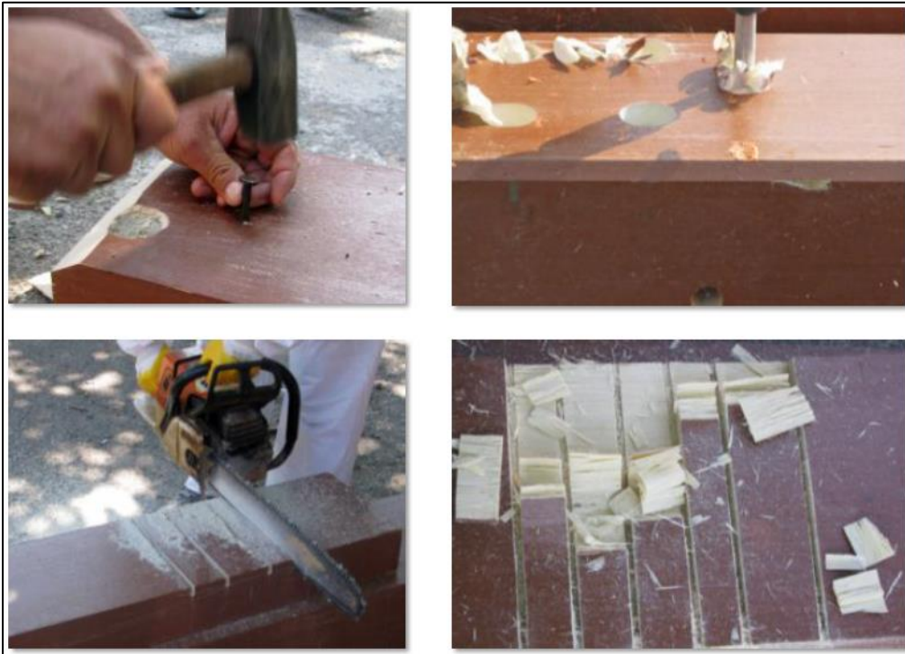
Photo 6. The FFU waybeams handle similarly to timber waybeams. The FFU material can be machined or worked using the same methods and tools as those used for timber sleepers.
