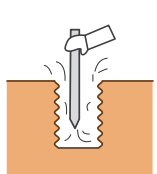
Cleaning bore hole
